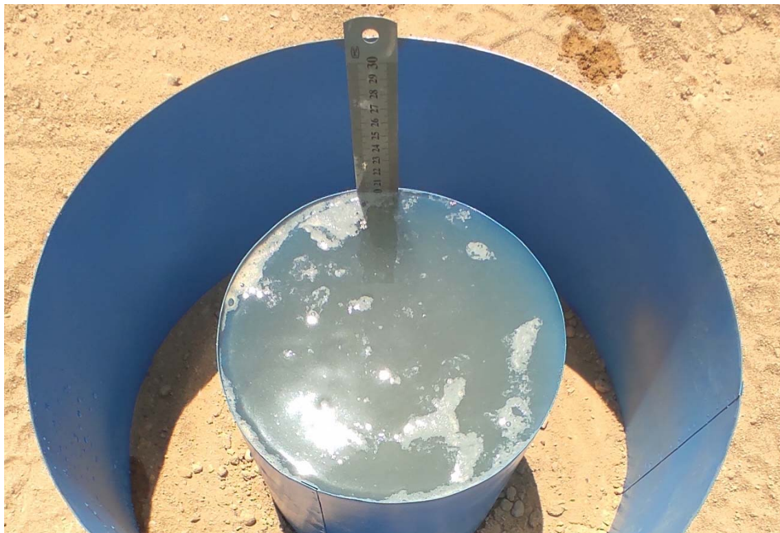
Fig. 13: Permeability Test in progress
