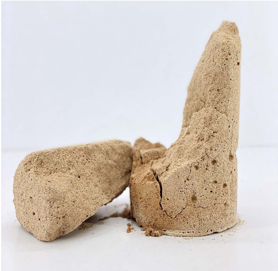
Fig. 17: Sample N.5 after Compressive Test
