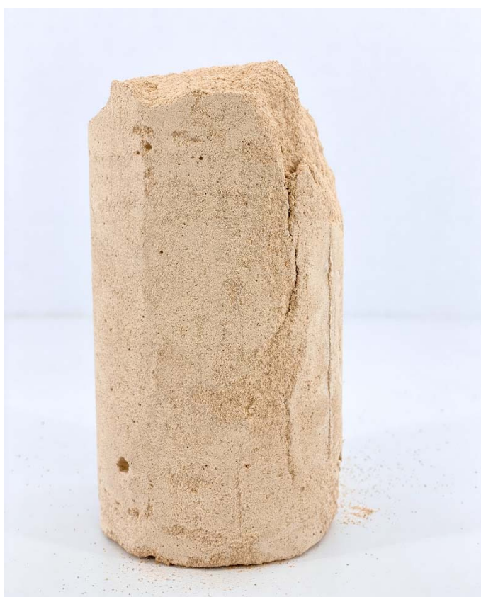
Fig. 15: Sample N.4 after Compressive Test
