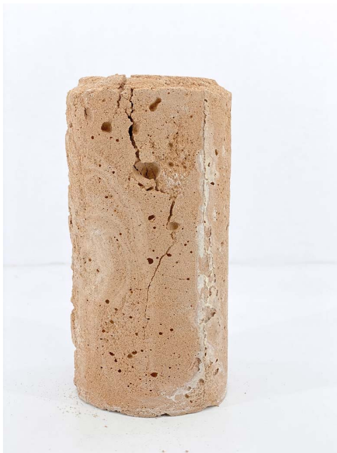
Fig. 21: Sample N.7 after Compressive Test
