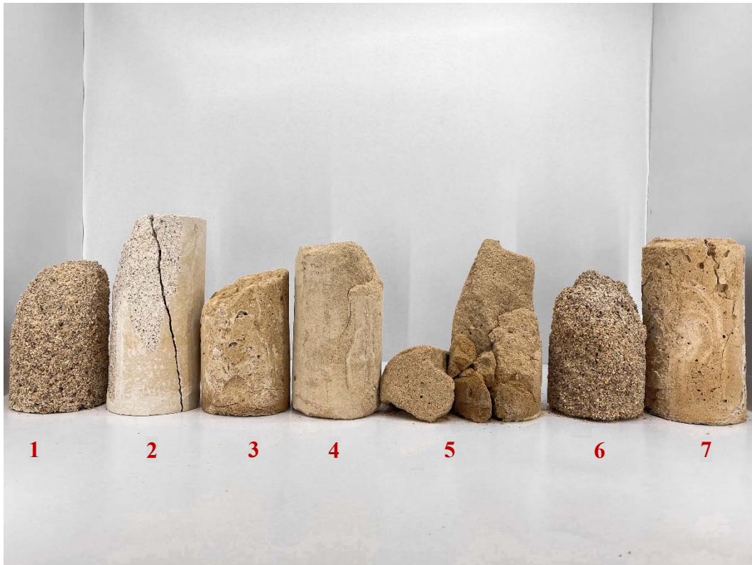
Fig.26: All Samples after Compressive Test
