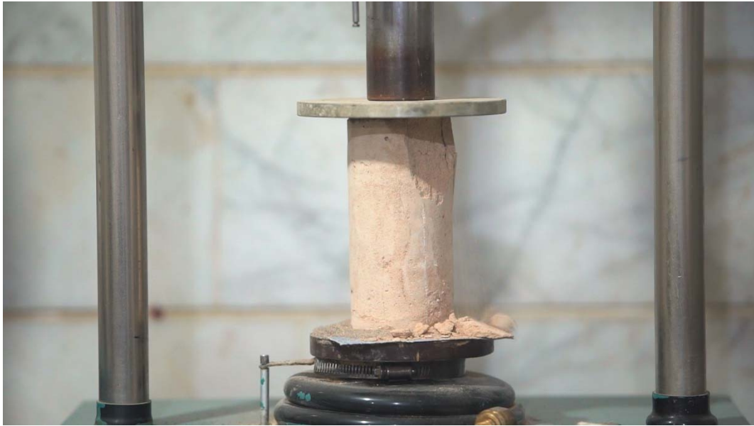
Fig. 24: Sample N.4 during Compressive Test
