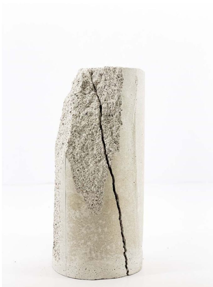
Fig. 11: Sample N.2 after Compressive Test
