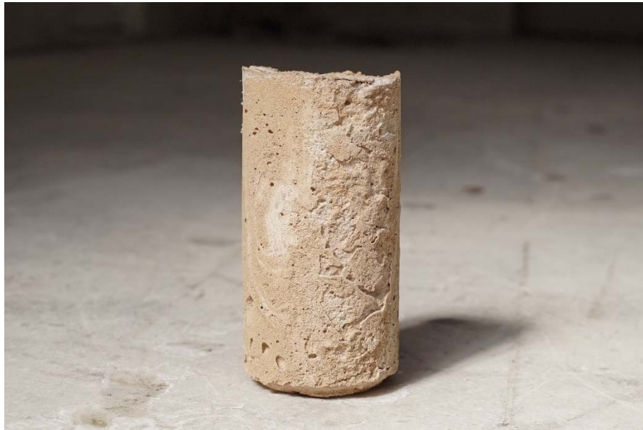
Fig. 12: Sample N.3 before Compressive Test
