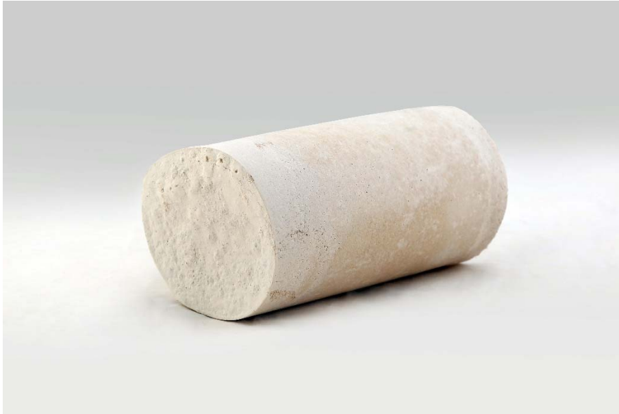
Fig. 10: Sample N.2 before Compressive Test
