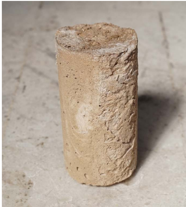
Fig. 16: Sample N.5 before Compressive Test
